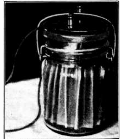
THIS electrolytic condenser was formed at 7.5 volts and its capacity is over 3000 mfd. It is used as a ripple remover in an A battery substitute.
